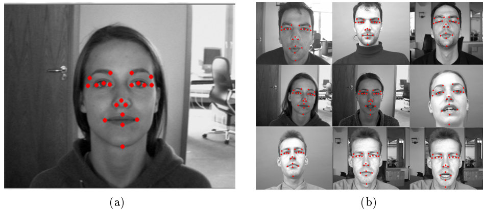
Figure 2.9: BioID database. (a) A total of 20 facial points are annotated including eye's points. (b) Each participants performs different conditions (user-sensor distance, head pose changes and illumination variation) to introduce variability in terms of appearance.
