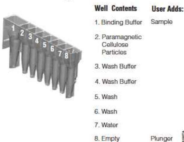
Figure 1. Maxwell® 16 LEV DNA Purification Cartridge. This figure shows the contents of a cartridge. In all cases, lysate sample is added to well # 1.
