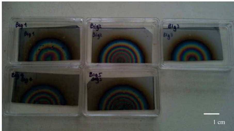
Fig. 3-1 Photo of silicon-supported TiO 2 thin films (from B1 to B5) made at PECVD T_s = 50, 100, 150, 200 and 250 °C respectively.
