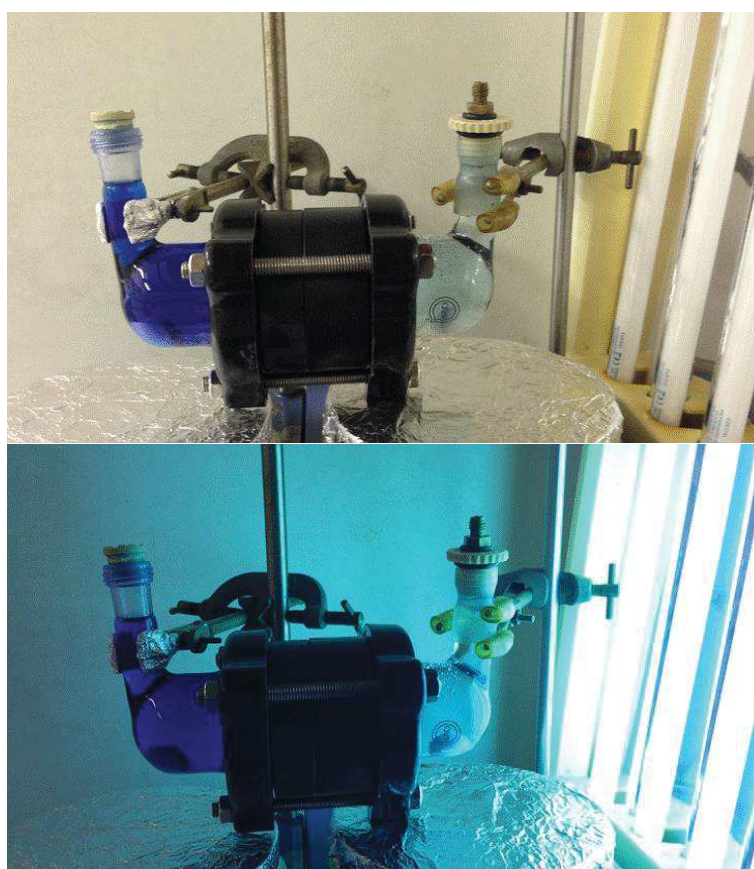
Fig. 2-16 Photos of the diffusion test with UV lamp off (up) and on (bottom).
