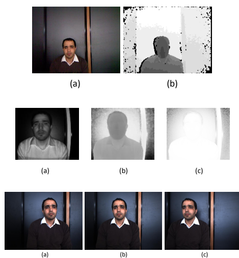
Figure 3.21 – Sample images from the 3 sensors. Top row: infrared sensor images from Kinect: (a) color (b) depth. Middle row: time-of-flight sensor images from SR4000: (a) infrared (b) depth (c) confidence matrix (bright pixels mean high confidence). Bottom row: image triplets from the stereo camera Bumblebee XB3.
