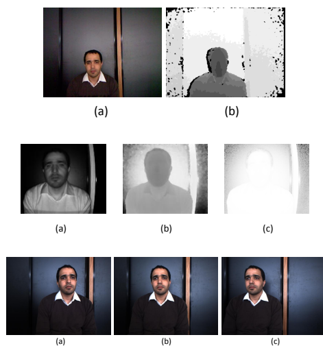
Figure 3.21 – Sample images from the 3 sensors. Top row: infrared sensor images from Kinect: (a) color (b) depth. Middle row: time-of-flight sensor images from SR4000: (a) infrared (b) depth (c) confidence matrix (bright pixels mean high confidence). Bottom row: image triplets from the stereo camera Bumblebee XB3.
