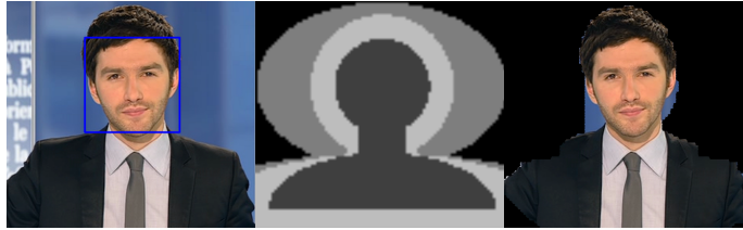
Figure 3.32 – Example of person extraction process on a single frame and a single person. Left: Original frame with the detected face. Center: Mask calculated from the detected face. Right: Result of the Grabcut algorithm applied on the original image using the mask.
