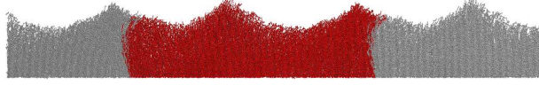
Figure 6.3: A snapshot for a larger studied systems ( L_x = 180 , L_y = 5 and L_z = 150 ) with a surface wave with multiple crests of wavelength L_x/2 \approx 90 ( Wi = 340 ). Again, we show the central box (in red) and the two nearest replicas (in grey) to highlight the wave periodicity.
