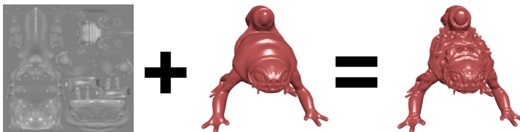
Figure 1.10 – Displacement Mapping — A detailed mesh (right) decomposed into a low-frequency mesh (middle) and a offset function (left) defined over the surface of this mesh.
