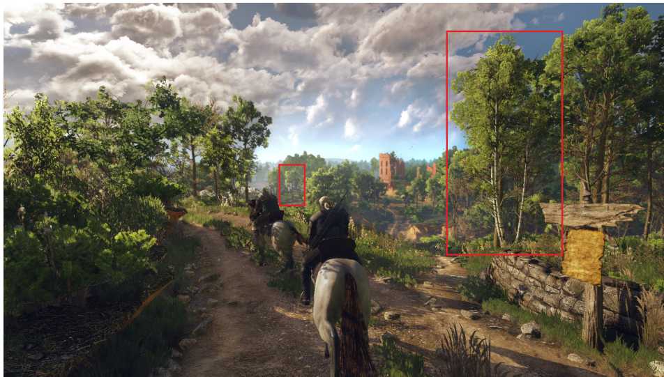
Figure 4 – Level of details in “The Witcher 3” — The resolution of the trees is adapted according to the view distance to reduce the complexity of the scene.
