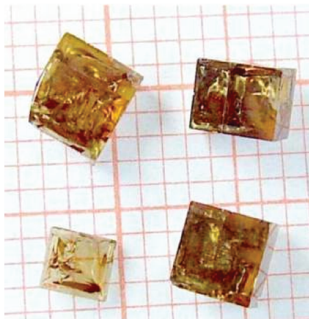
Figure 2.5: 0.68PMN-0.32PT single crystal (placed on millimetre paper) [Luo et al., 2009].
