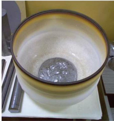
Figure 2.4: A ceramic crucible used in crystal growth.
