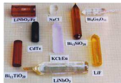
4) Other single crystals grown using the same method (all over 20mm in diameter)
