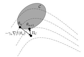
Figure 1-3 – Projected subgradient. We denote by  $\Pi_{\mathcal{C}}$  the Euclidean projection on the convex set  $\mathcal{C}$ .
