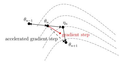
Figure 1-2 – Accelerated gradient descent.
