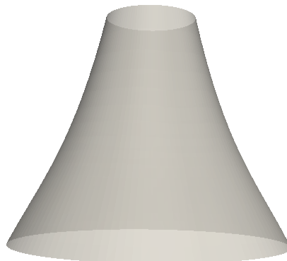
Figure 5.30 Optimal shape for the joint anisotropy and shape design of the holed circular plate.
