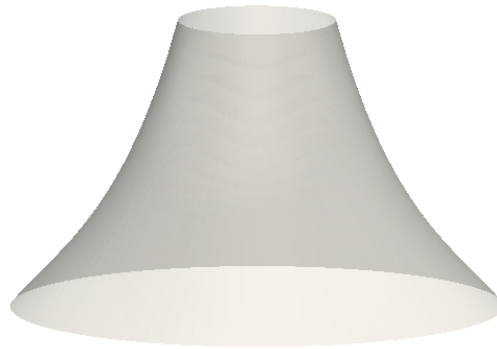
Figure 5.21 Shape design: Optimal shape corresponding to the holed circular plate under edge load.
