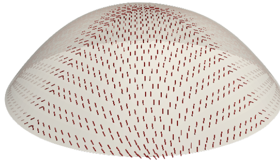
Figure 5.15 Anisotropy and shape design: Optimal orthotropy direction field of the optimal design corresponding to the circular plate under weight-load.
