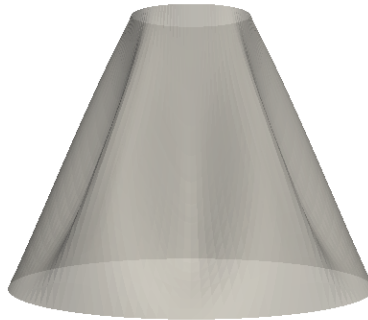
Figure 5.25 Shape design with anisotropy material with an orthotropy angle \Phi_1 = \frac{\pi}{4} : Optimal shape corresponding to the holed circular plate under edge load.
