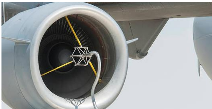
Figure A-1: Full-scale test of volcano particle intake performed by NASA [145]
