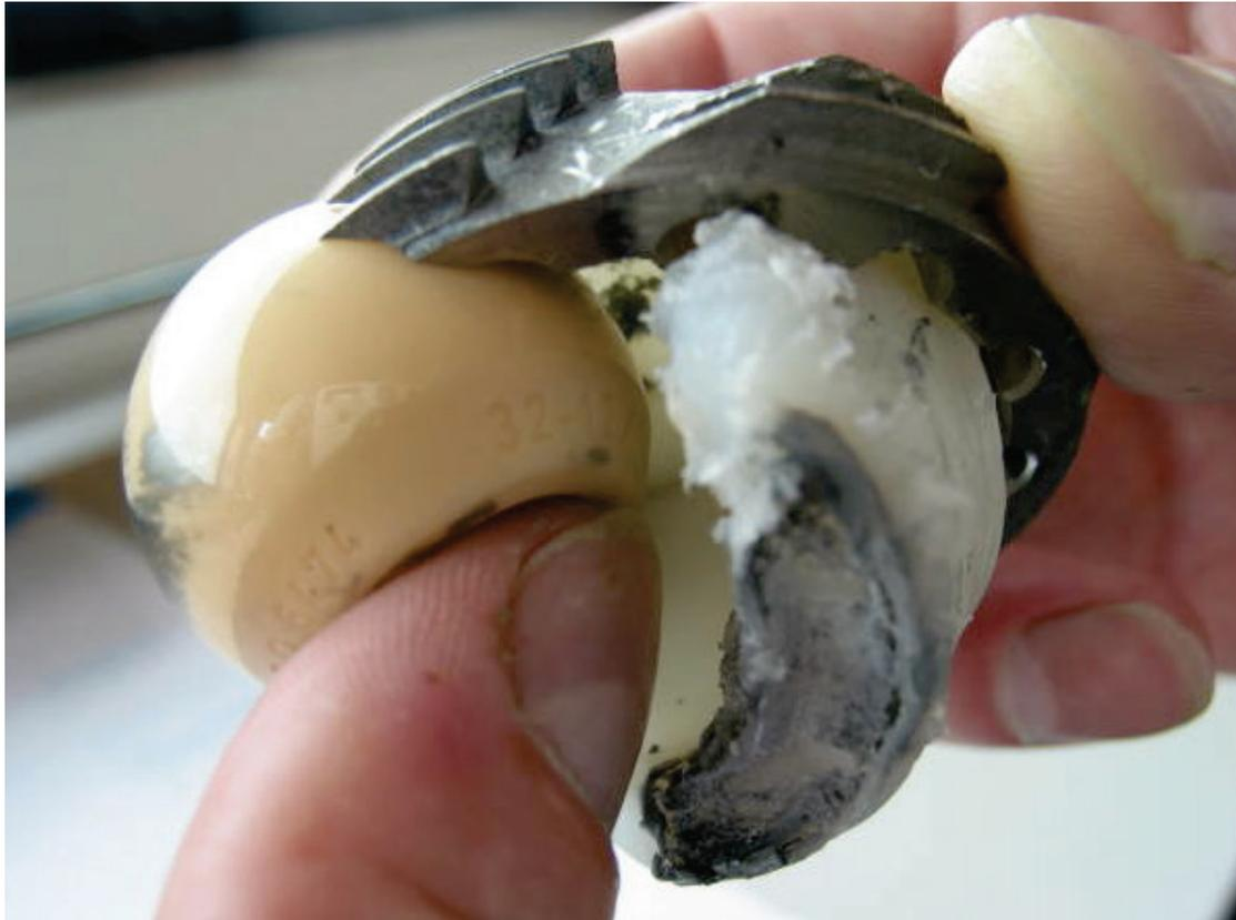
**Figure 1.9.** Ceramic-on-Polymer joint. The ceramic ball head wore the liner and even continued through the metallic shell. (Source: Dr. med. Karl-Heinz Günther, [www.doccheck.com](http://www.doccheck.com))
