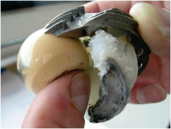
**Figure 1.9**. Ceramic-on-Polymer joint. The ceramic ball head wore the liner and even continued through the metallic shell. (Source: Dr. med. Karl-Heinz Günther, www.doccheck.com)
