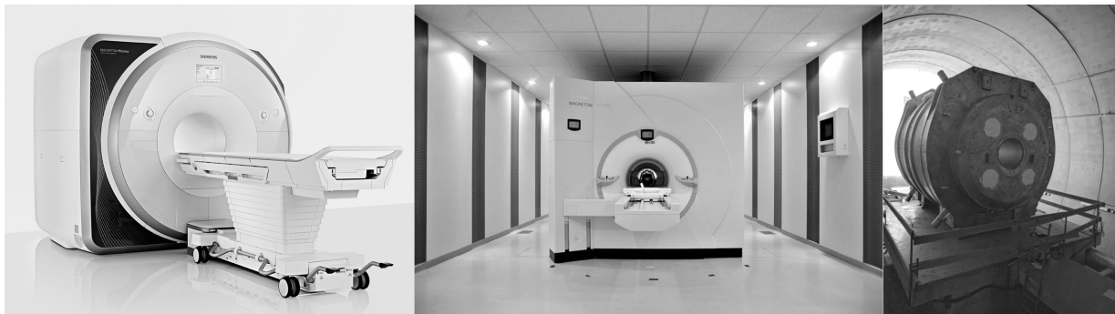
Figure 2.2: NeuroSpin's 3 T PRISMA-fit (left) and 7 T MAGNETOM (center) MR Scanners (Siemens Healthcare, Erlangen, Germany) plus a peak at the "naked" 11.7 T Iseult magnet (CEA-IRFU) (right).
