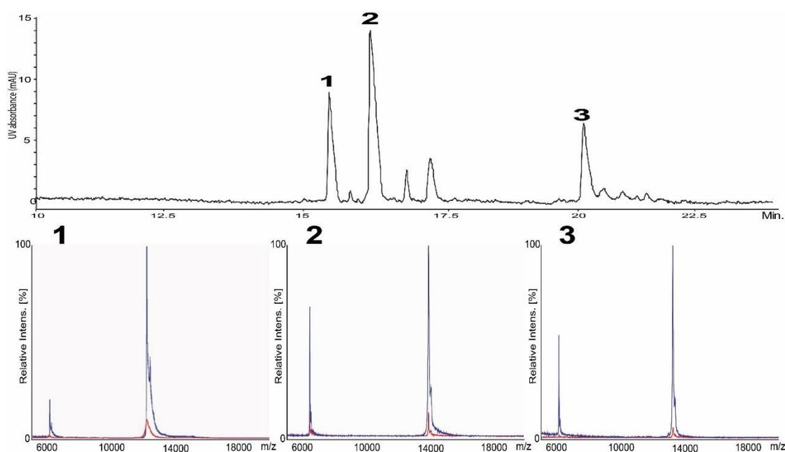
**Fig. 2.** UV Electropherogram with fraction collection and MS spectrum of (1) Cyt c, (2) Lys and (3) RNase A from CE-UV/MALDI-MS analysis. (Red spectrum) single deposition on the MALDI target-plate.(Blue spectrum) Enrichment of three repetitions on the same MALDI target-plate
