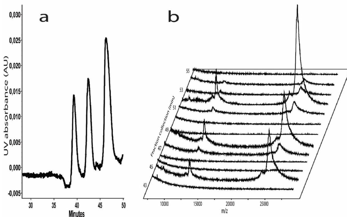
**Figure 2.** CZE-UV off-line coupled to MALDI-MS via fractionation for a middle-up characterization of Cetuximab  $Fc/2$  variants. (a) CZE-UV electropherogram. (b) Analysis of CZE-UV fractions by MALDI-MS. CE Experimental conditions: See Fig. 1; MS condition: See Experimental section; sample, IdeS digest of cetuximab ( $5 \mu\text{g}/\mu\text{L}$ )
