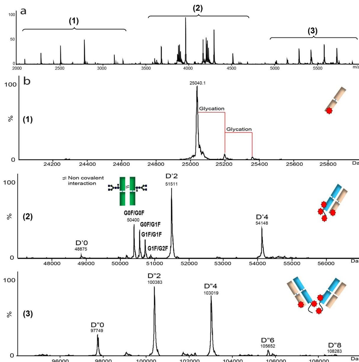
**Figure 2.** (a) MS spectra corresponding to Native MS NanoESI infusion of middle-up brentuximab vedotin. (b) Charge state deconvoluted mass spectra of (1) Lc-drug conjugated subunit, (2) Fab subunits with the incorporation of 0 to 4 payloads and Fc<sub>2</sub> homodimers and (c) F(ab)<sub>2</sub> subunits with the incorporation of 0 to 8 payloads.
