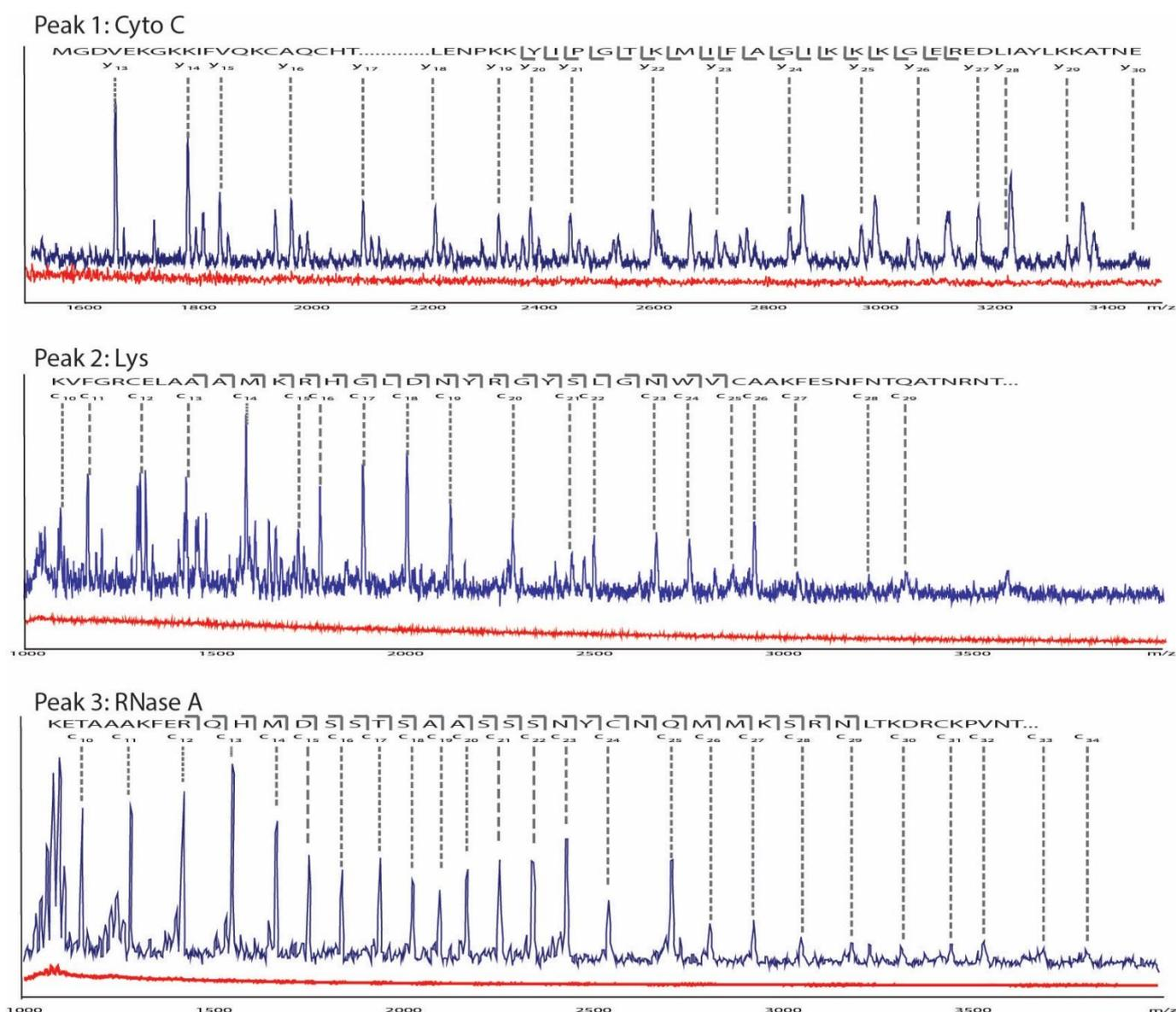
**Fig. 3.** Top-down MALDI-MS/MS spectra of Cyt c (peak 1), Lys (peak 2) and RNase A (peak 3) from CE-UV/MALDI-MS/MS analysis of a solution of three proteins with fraction collection (see Fig. 1). (Red spectrum) single deposition on the MALDI target-plate. (Blue spectrum) Enrichment of three repetitions on the same MALDI target-plate.
