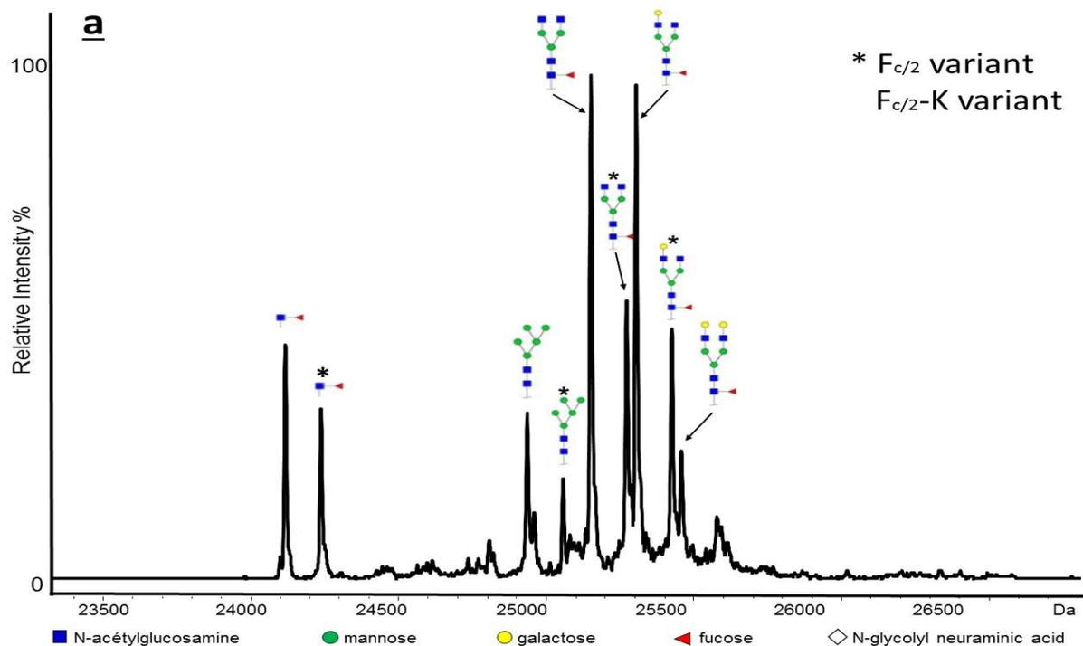
**Figure S-2.** (a) Off line CE-UV/ESI-MS separation of middle-up cetuximab charge variants. (b) Mass spectra corresponding to the 3 major peaks. Experimental conditions: Inlet BGE: EACA 200 mM acetate ammonium 25 mM pH 5.70 and outlet BGE: ammonium acetate 25 mM pH 5.70; other conditions: See Figure 1, MS Experimental conditions: See Experimental section; sample, IdeS digest of cetuximab (5 µg/µL); sample injection 0.5 psi 50s.
