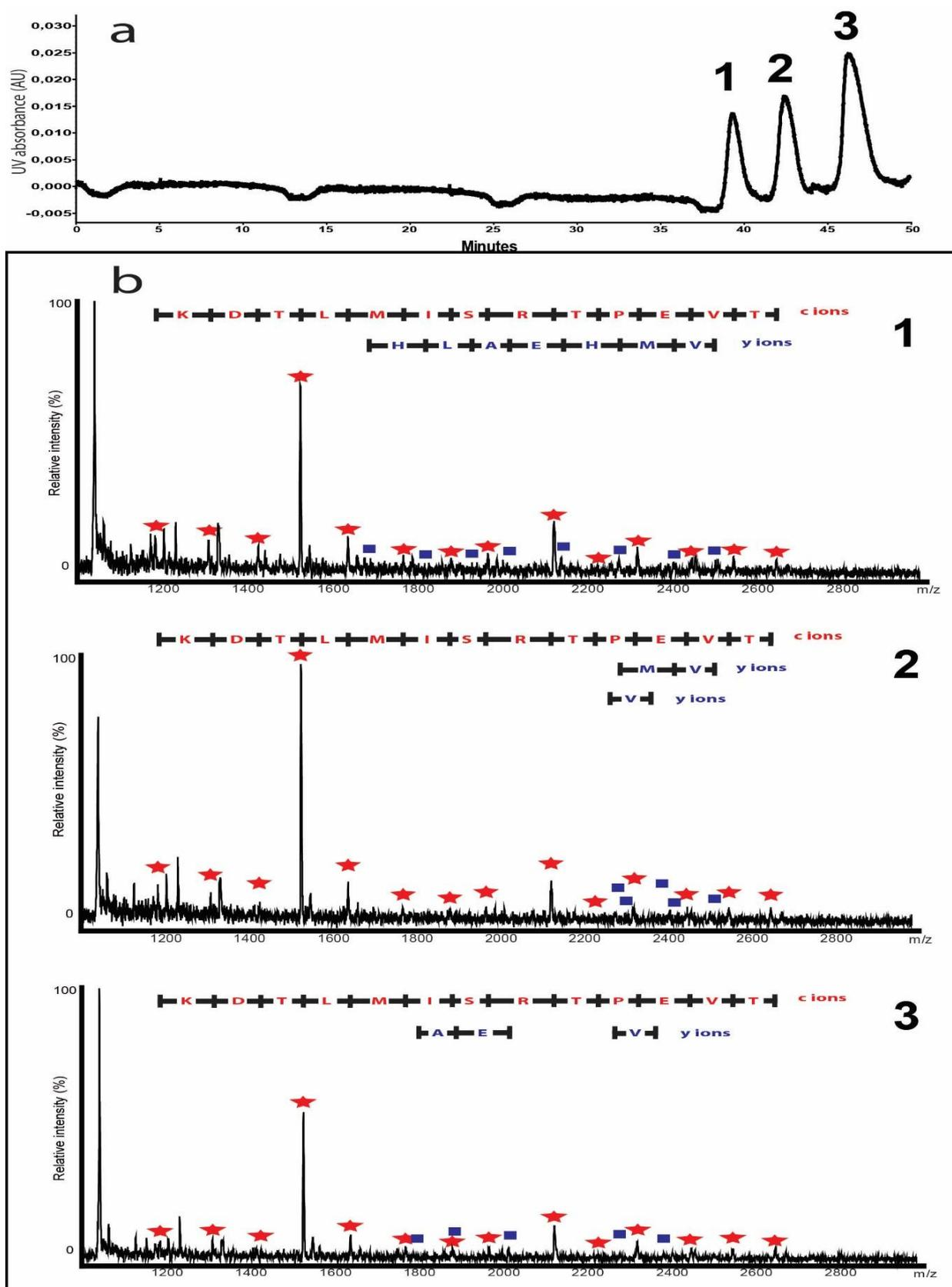
**Fig. 4.** CZE-UV off-line coupled to MALDI-MS via fractionation for a middle-up characterization of Cetuximab  $F_{c2}$  variants. (a) CZE-UV electropherogram. (b) Middle-down MALDI-MSD spectrum of  $F_{c2}$  variants corresponding to the three peaks. CE Experimental conditions: Experimental section; MS condition: See Experimental section; sample, IdeS digest of cetuximab (5 mg/mL); sample injection 0.5psi 60s.
