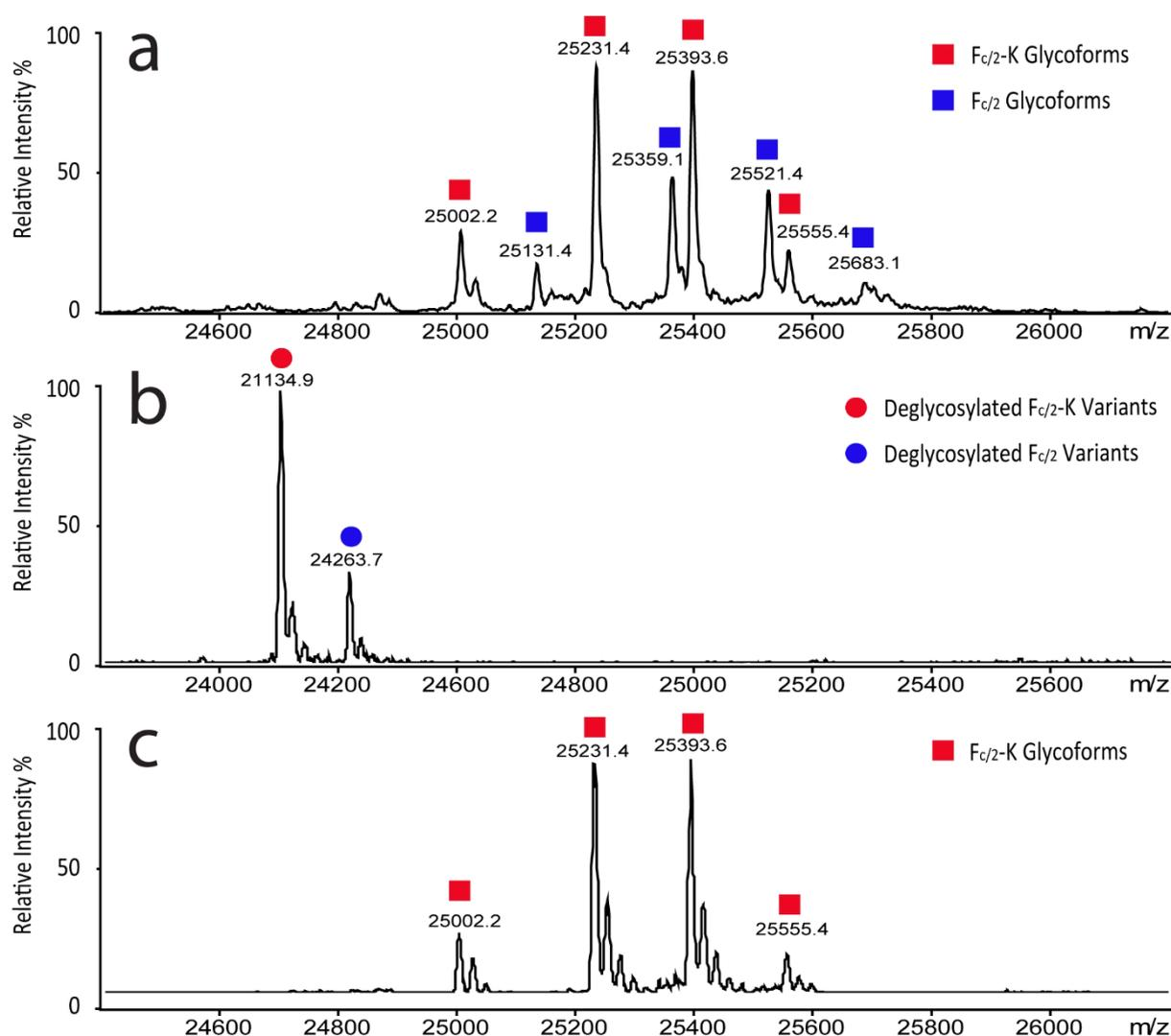
**Figure 4.** Fc/2 variants deconvoluted mass spectra of (a) IdeS digest cetuximab, (b) IgGZERO+IdeS digest cetuximab and (c) CP-B+IdeS digest cetuximab. Experimental conditions: 50%/49%/1%, acetonitrile/water/formic acid (v/v/v); sample concentration 1  $\mu$ M.
