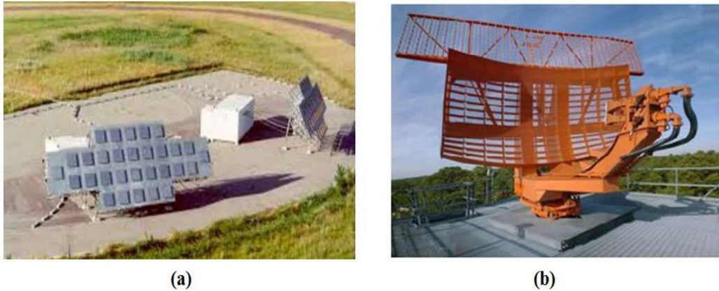
Figure I-3. (a) French radar designed to detect satellites orbiting between 400 and 1000 km, (b) primary mechanical scanning radar for an airport.
