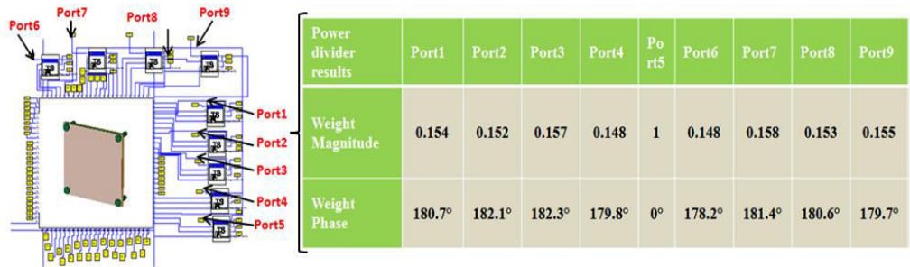
Figure V-8. “Case3” ARMA antenna connected to the polarization circuits fed by outputs of the realized power divider.
