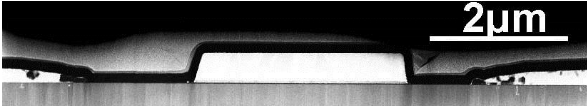
Figure 7.4: Geometry of a HEMT structure with its contacts. From left to right are the drain, gate and source. The source to gate length is shortest. The continuous large dark contrast indicates the SiN cap layer.
