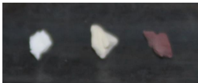
Figure 2-12: Pictures with the naked eye of the pristine porous P(GMA- co -EGDMA) monolith (white, left), of the same monolith after impregnation with gold salt precursor solution (yellowish, middle) and of the monolith loaded with Au nanoparticles after complete reduction of \text{Au}^{3+} cations under \text{Ar}/\text{H}_2 (v/v : 95/5) stream at 100 °C during 24 h (wine red, right).
