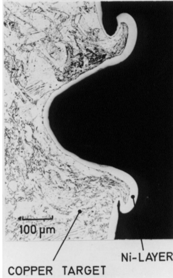
Figure 3.3: Crater produced in copper by a focused Nd laser beam of an energy of 10 J and a duration of 10 ns. From [36]
