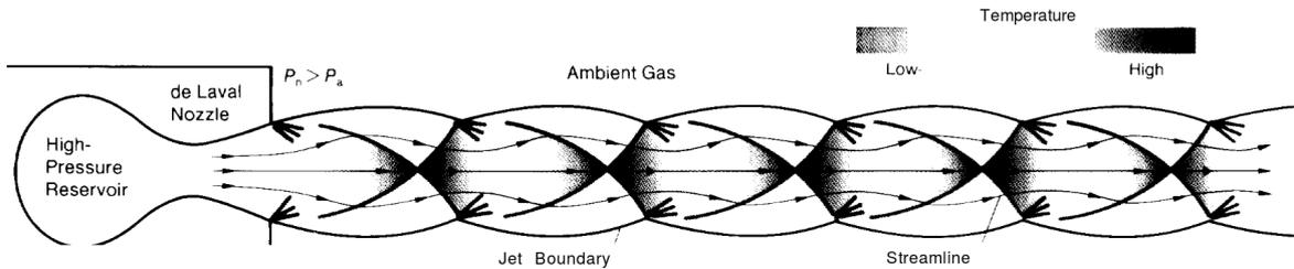
Figure 4.3: From [2]. Idealized supersonic slightly underexpanded jet ( $P_{jet} > P_{background}$ ). Conical shocks are formed at regular steps as a consequence of the action of the background on the jet material.
