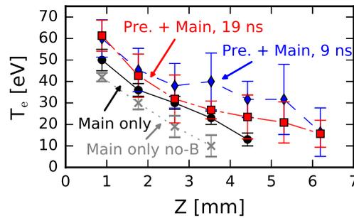
Figure 6.3: X-ray spectrometry measurements of  $T_e$  from the FSSR. Lines with circles (and X's) represent the main pulse alone with (and without) an applied 20 T B-field. Lines with diamonds and squares show cases with a precursor of 9 and 19 ns delay, respectively.
