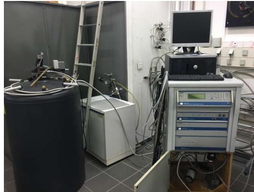
Figure 2. 9. The Quantum Design PPMS device used for heat capacity and resistance measurements.
