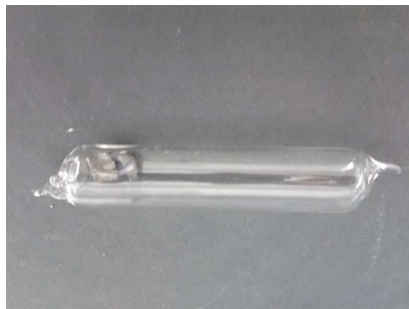
Figure 2. 4. Sample sealed in an evacuated quartz ampoule for thermal treatment.
