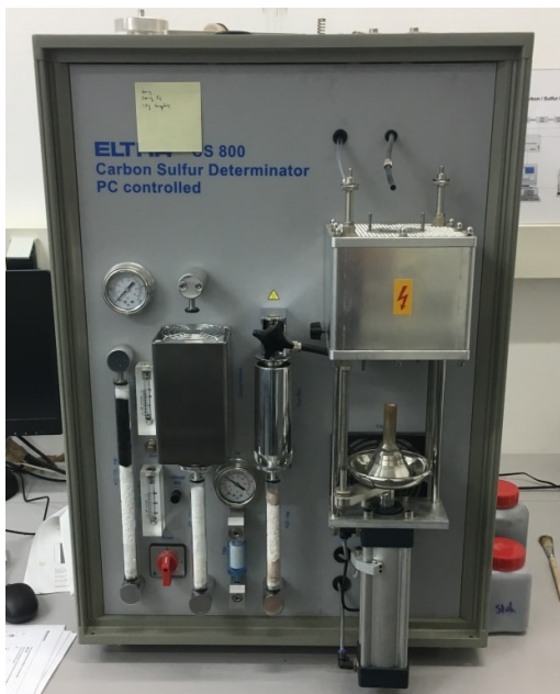
Figure 2. 11. Eltra CS800 carbon/sulphur determinator used to dose the carbon content.
