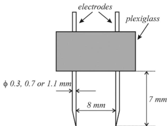
Figure 2.1: Needle electrodes used in experiments of [110].
