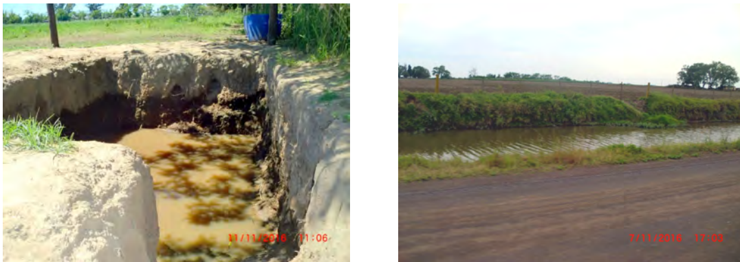
Figure 3.8 – Pictures taken at Monte Buey during the Cal/Val campaign in November 2016 that illustrate the water table level (left) and the trenches built for water drainage (right)
