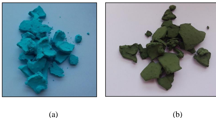
Figure 4- 2 Precursors after drying (a) and catalyst after calcination at 400 °C (b)
