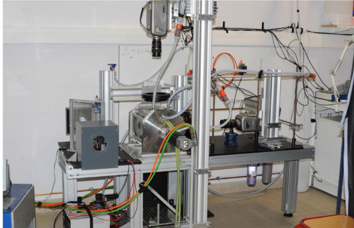
Figure 2.1: Photograph of the S-PTV setup used to study the von Kármán Flow.
