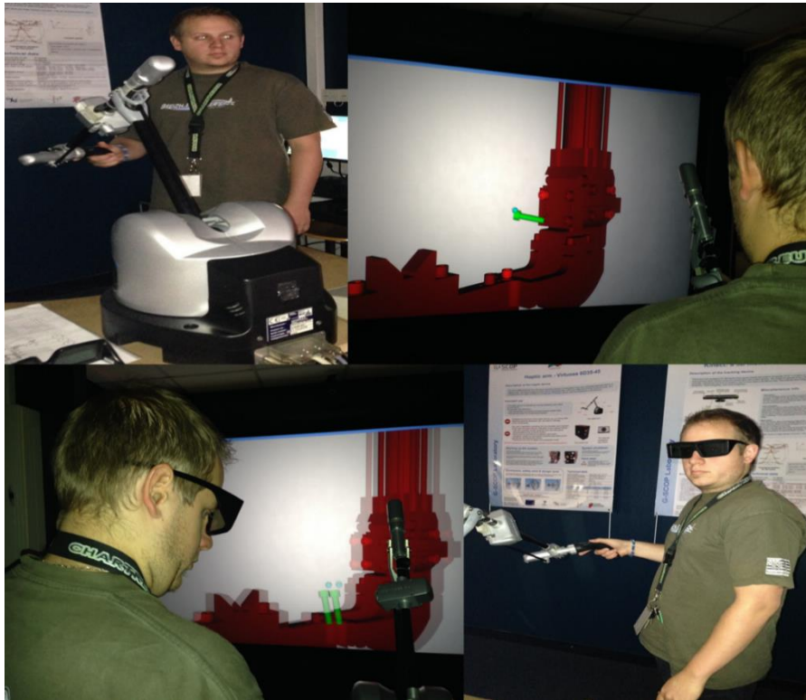
FIGURE 2-3 A participant interacts with the collaborative virtual environment either in 2D or 3D and either with or without force feedback
