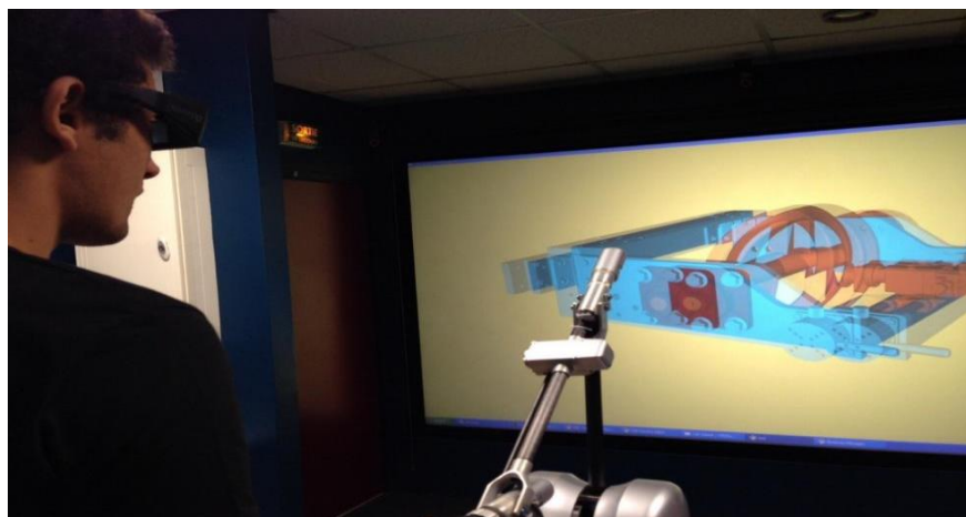
FIGURE 5-7 The participants work in a comfortable stand postures by the use stereoscopy with force-feedback to manipulate the mechanism
