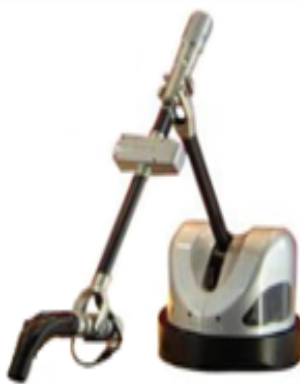
FIGURE 2-4 A haptic arm interface is a haption Virtuose 6D35-45
