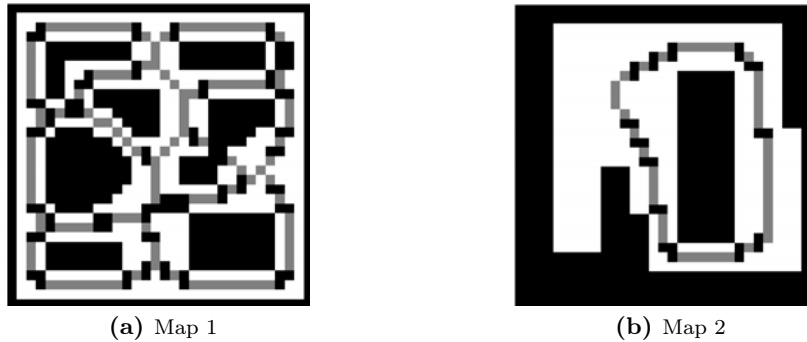
Figure 6.9: Thin skeleton computed by an Area Voronoi Diagram.
