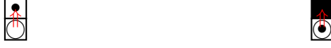
Figure 2.1: This figure illustrates the deterministic position outcome p' ( \bullet ) obtained after applying action up ( \uparrow ) from position p ( \circ ) on any local occupancy map m_{loc} . Formally, we illustrate the position p' of the successor state from the predecessor s and the action a : s' = (p', m_{loc}, c') = TransitionModel(s = (p, m_{loc}, c), \uparrow) . The example on the left represents a local occupancy map with two cells that are free of obstacles (white); the robot stands on the bottom cell ( \circ ) and ends up in the top cell ( \bullet ) by moving up ( \uparrow ). On the right example, the top cell is occupied by an obstacle (black), hence the robot remains in the bottom cell when deciding to move up. Similar patterns can be obtained for other moving directions under rotational symmetry.
