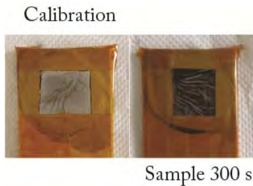
Figure 3.2.7. Photo of a) calibrate and b) sample for 300 s electrodeposited membranes of 30 nm of pore size.
