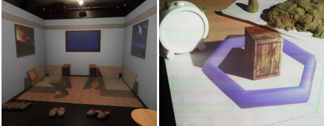
Figure 83: Spatial immersive augmentation: Square CAVE (left), dynamic perspective-corrected projection over an arbitrary environment (right, the box and the bluish hexagon are projected)
