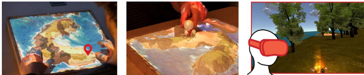
Figure 57: users can shape the terrain with their hands (left), chose a location (centre) and then immerse themselves thanks to an HMD (right). Biofeedback is present at all times, gently influencing the mini-world.
