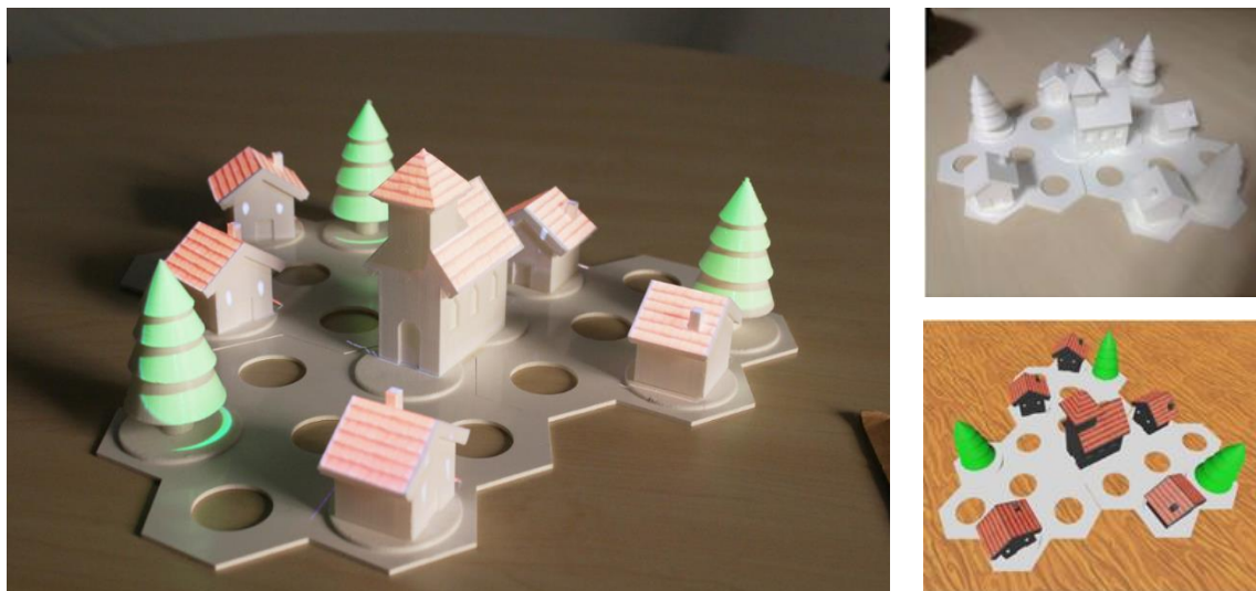
Figure 13: Texture mapping (left) is the result of combining physical (right-top) and digital (right-bottom) counterparts with the same geometry. In this case it is performed using projectors, but it would also be possible to use screens or LEDs placed onto the augmented objects.
