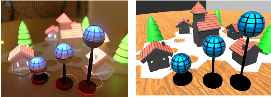
Figure 35: SAR (left) and VR (right) versions of the mock-up and the targets (3, 6, and 9cm in height)
