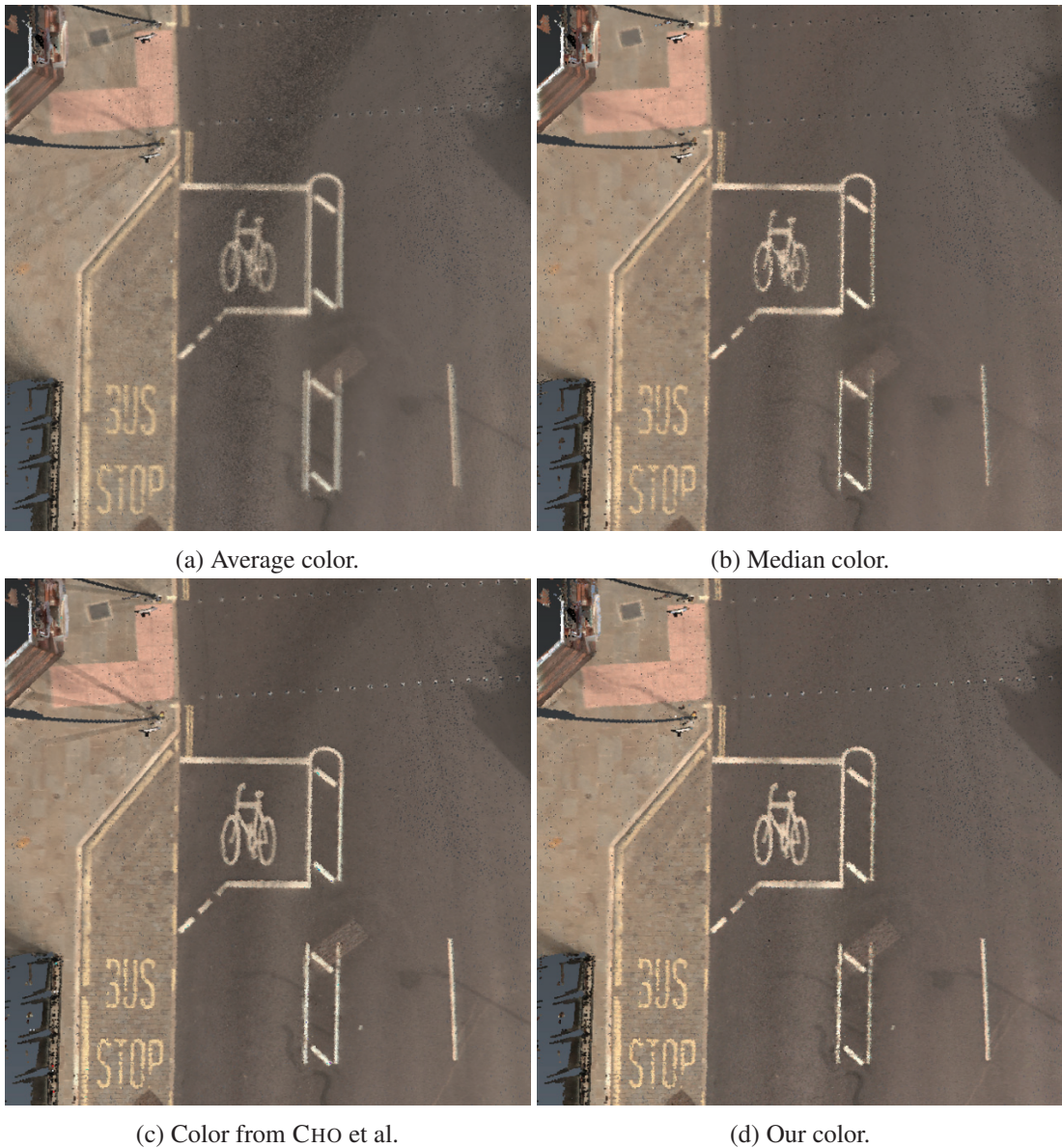
Figure 4.7: Top view of the colored point cloud in Castle street near the train station. Average and median color are blurry compared to other colorization methods. Stains of the traffic light pole are visible on the top left part of Figure 4.7(a) and Figure 4.7(c).
