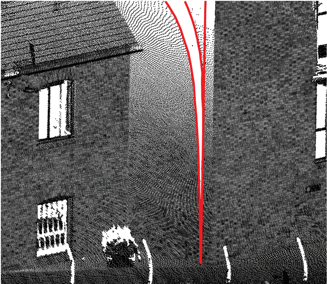
Figure 1.5: Top-down rendering of a continuous scan performed with a vehicle mounted LiDAR in 3DReshaper. The rotation axis of the LiDAR was inclined which created particular oblique occlusion areas visible on this rendering.
