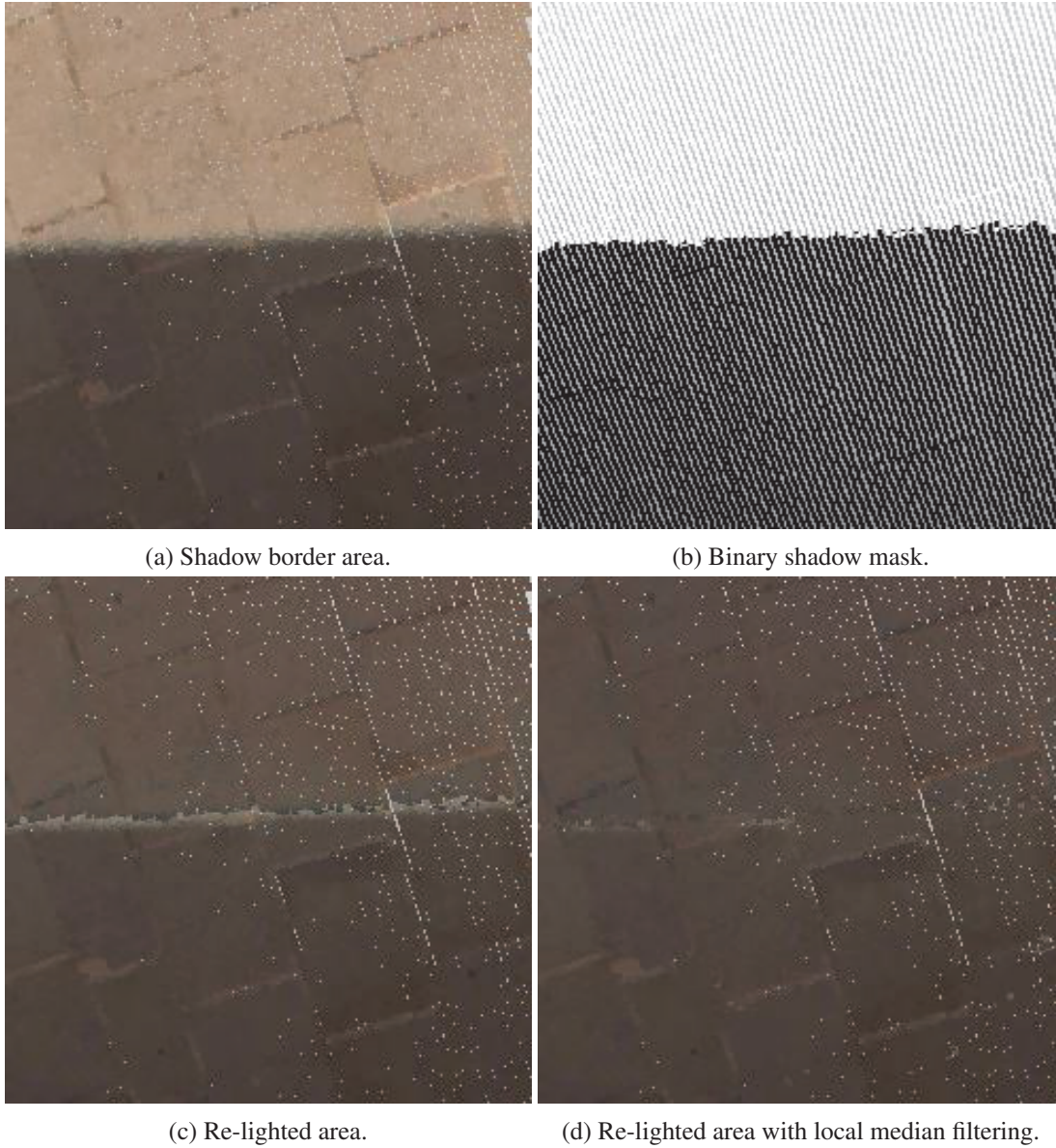
Figure 4.14: Small penumbra zones on the boundary of a shadow can have non negligible effect when re-lighting a point cloud. A simple median filtering of points located on the boundary of the shadow mask mitigate the apparition of artifacts.
