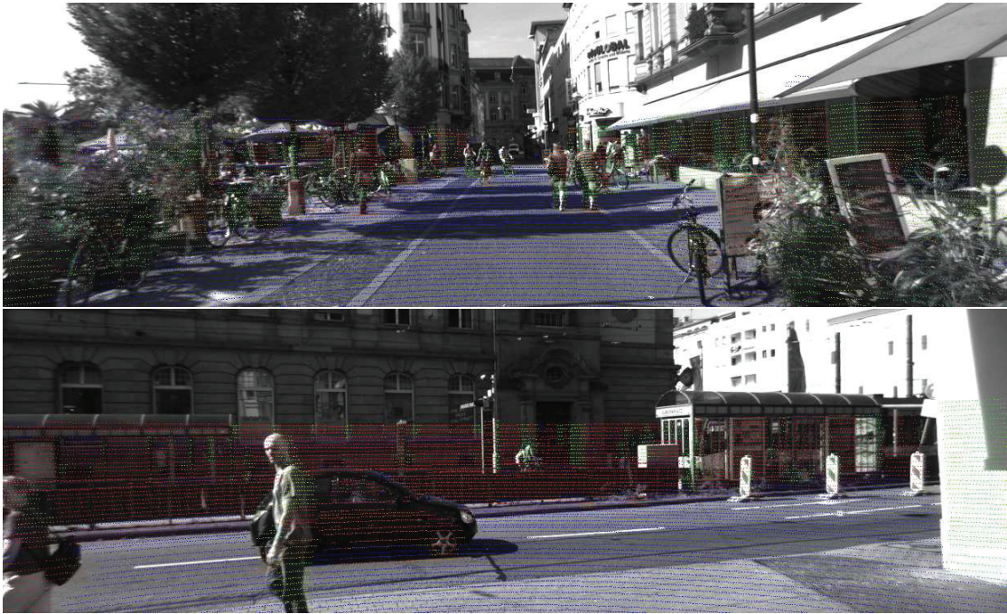
Figure 3.11: Projection of the point cloud on two of the images of the Kitti dataset containing image/scan pairs. The Velodyne LiDAR point cloud is sparse, and its scanning height is limited, which only offers a small amount of corresponding data.
