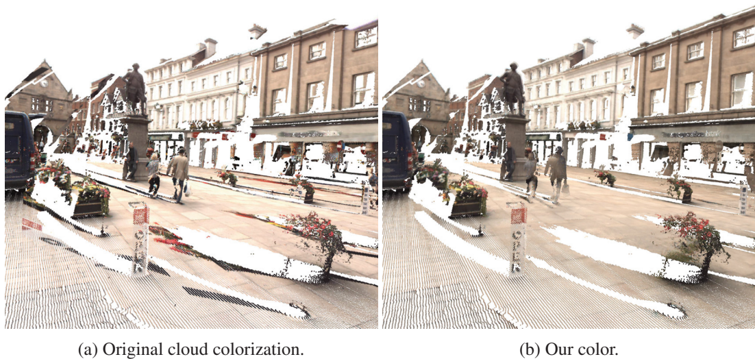
Figure 4.10: Image view of the square around the Statue of the Major-General Robert Clive. Original colorization has several artifacts around static occluding objects that were successfully removed. Other artifacts on building walls were also removed by our recolorization.
