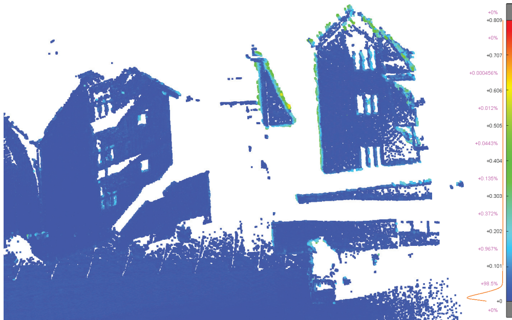
Figure 5.8: Visualization of the distance between the new upsampled points and their closest neighbors in the original point cloud.
