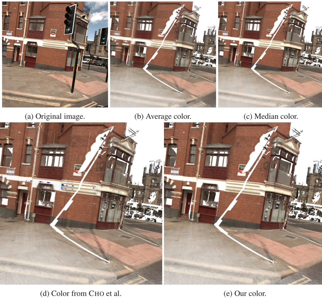
Figure 4.8: Views of the colored point cloud in Castle street near the train station. An interpolation has been performed to improve the visibility. In Figure 4.8(d) the traffic light pole color is projected onto the ground and the wall, mixed with the proper color of the surface, whereas it is not present in Figure 4.8(e).
