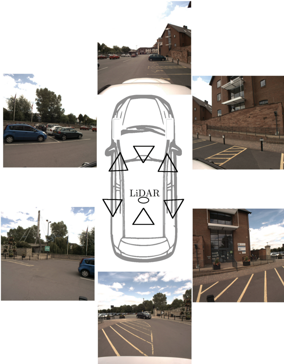
Figure 1.8: The 6 images of the environment acquired every meter along the acquisition path of the Pegasus II scanning device. All images contain an important overlap. Original car outline is from the Kitti dataset presentation article [Gei+13].
