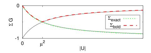
Figure 6: The two branches of the self-energy  $\Sigma$ , multiplied for convenience by G, as a function of the interaction strength |U|, for fixed  $\mu$ . Dotted line: exact self-energy  $\Sigma_{\text{exact}} = \Sigma(\mu, U)$ , dashed line: bold series  $\Sigma_{\text{bold}}(G, U)$ . The upper branch corresponds to  $\Sigma^{(+)}(G, U)$ , the lower branch to  $\Sigma^{(-)}(G, U)$ . Here, G stands for the exact  $G(\mu, U)$ .
