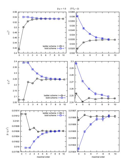
Figure 2: Dimensionless density  $n\lambda^3$ , contact parameter  $\mathcal{C}\lambda^4$ , and inverse orderparameter susceptibility  $\beta/(\chi\lambda^3)$  as a function of maximal order of expansion  $\mathcal{N}$ , for  $\beta\mu = -1.5$ , where  $\lambda = \sqrt{2\pi\beta}$  is the thermal de Broglie wavelength.
