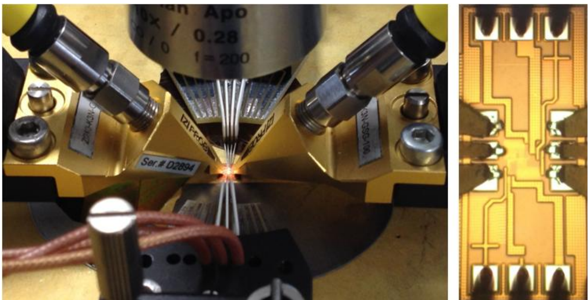
Figure 4.1 – RF wafer probe station and chip under measurement
