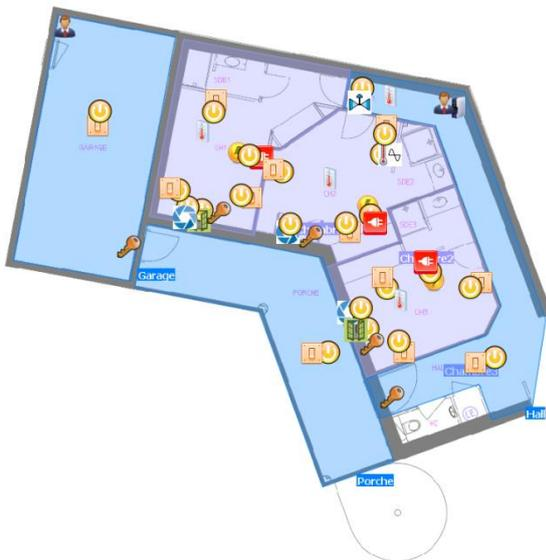
**Figure D-5: Sensors distribution for ground floor bedrooms and garage**
