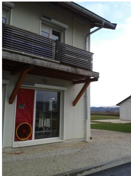
**Figure 3-9: Blower-door test, for the I-BB house**
