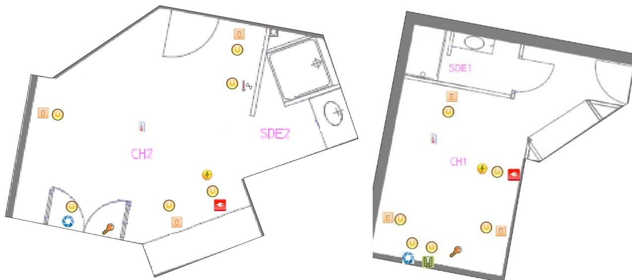
Figure D-6: Sensors distribution for a ground floor bedroom: room2 (CH2) and room 1 (CH1)
