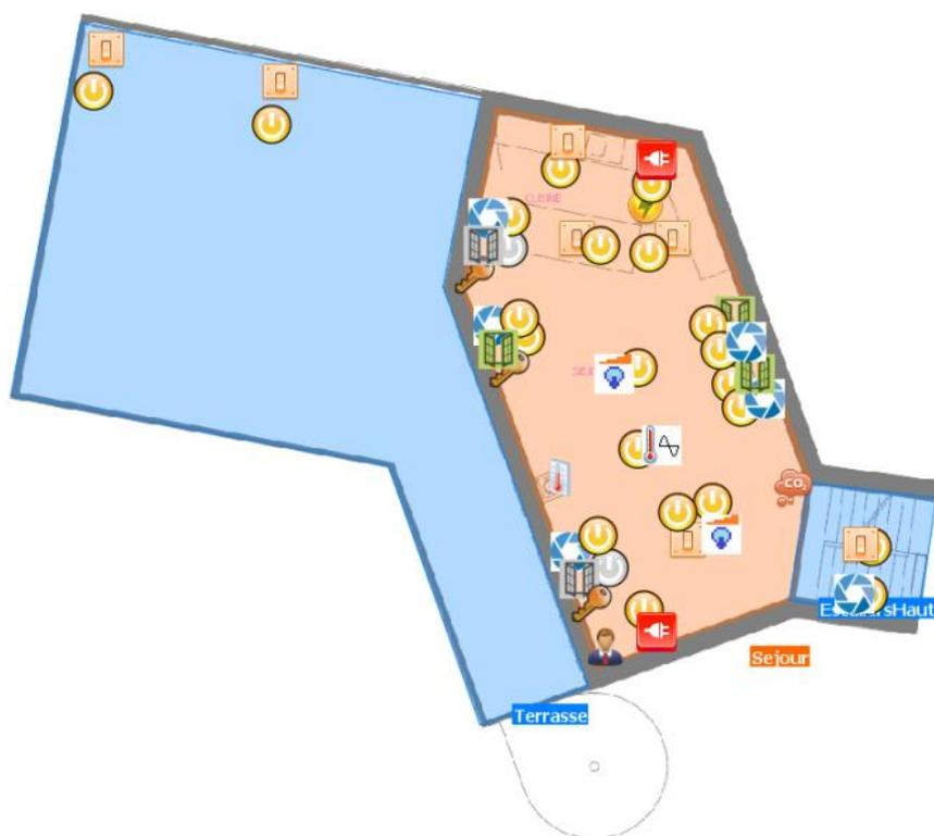
Figure D-9: Sensors distribution for the living room
