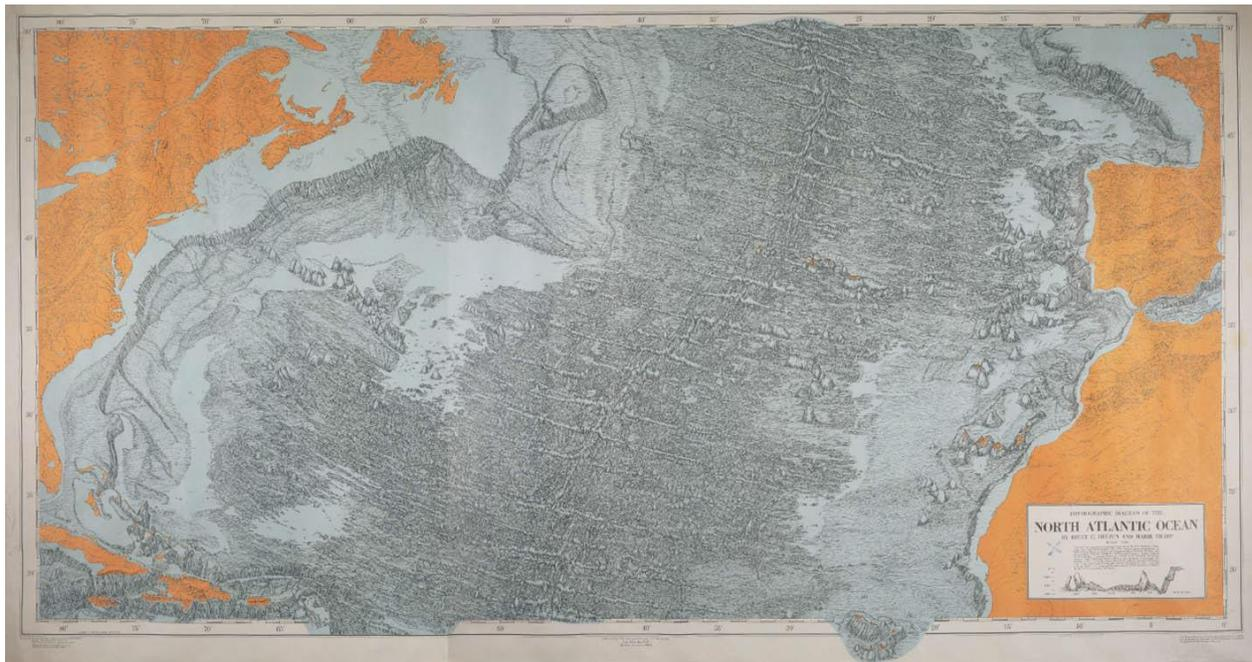
*Figure 1.2. Marie Tharp's first bathymetric map, based on echo-sound data acquired by research vessels after World War II, during the Cold War. At the centre of the ocean, there is a clear feature visible, which is nowadays known as the Atlantic Mid Oceanic Ridge (Heezen et al., 1959).*
