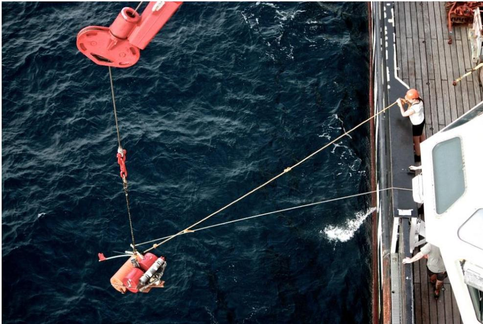
*Photo 5. Deploying OBS stations. Every 12-15 kilometres an OBS station is thrown overboard. With the anchor positioned correctly, they should reach the bottom in little time. It is important that the anchor sinks well into the sediments, because only then will the geophone record the refracted and reflected waves produced by the airguns. (Photo by Menaka Goonewardena, 2017)*
