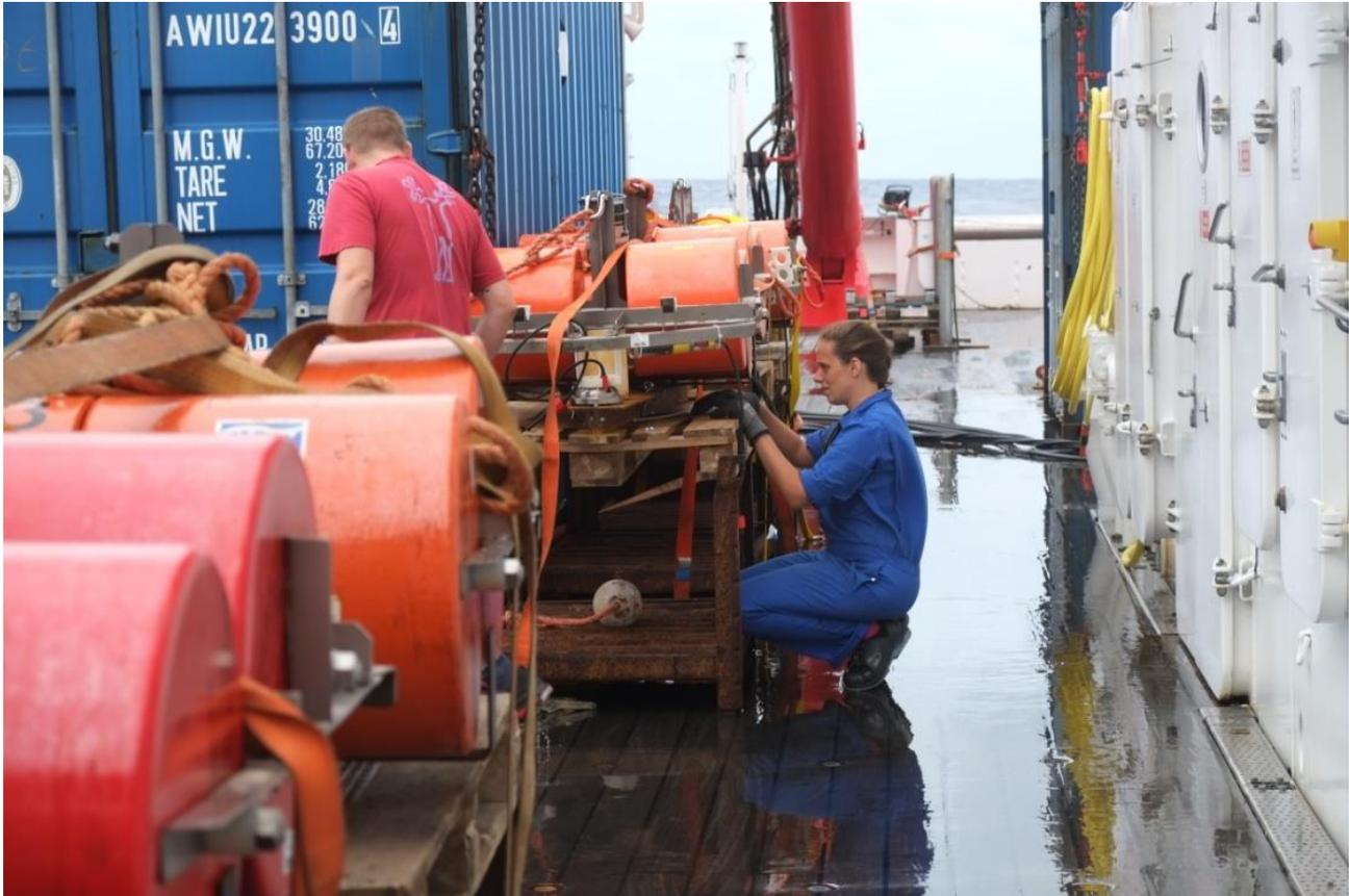
*Photo 3. Preparing the OBS stations on deck. Releaser, flash light, radio beacon, pressure tube, hydrophone and geophone are all attached to the floating device that is again attached to an anchor, before deployment. (Photo by Mareen Lösing, 2017)*
