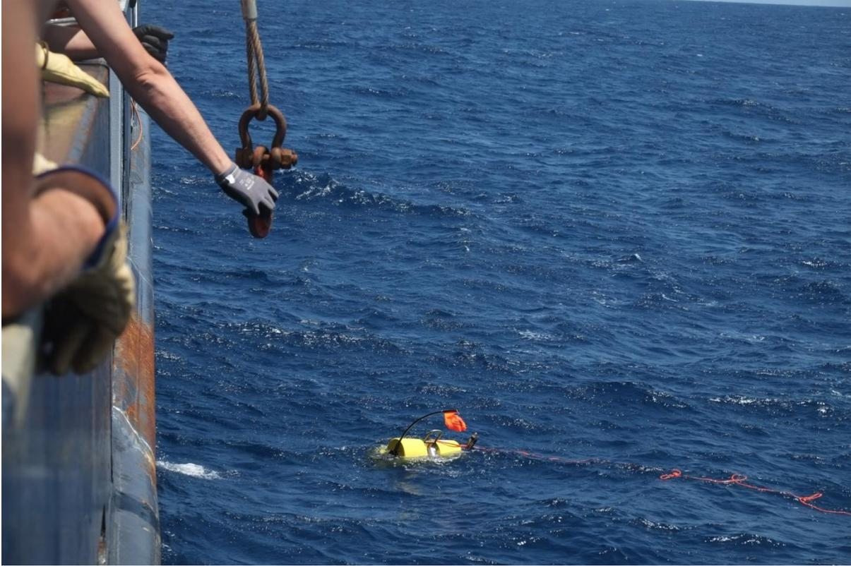
*Photo 8. OBS recovery. The OBS rises with 0.9 m/s to the surface. With a depth of over 4300 meters, the ascent takes roughly 80 minutes. When there are strong currents, heavy waves or bad weather they are not so easy to spot. Luckily the OBS station is equipped with a radio beacon and when they reach the surface the radio picks up the signal. They also have a flash light so it can be easily spotted at night (Photo by Mareen Lösing, 2017)*
