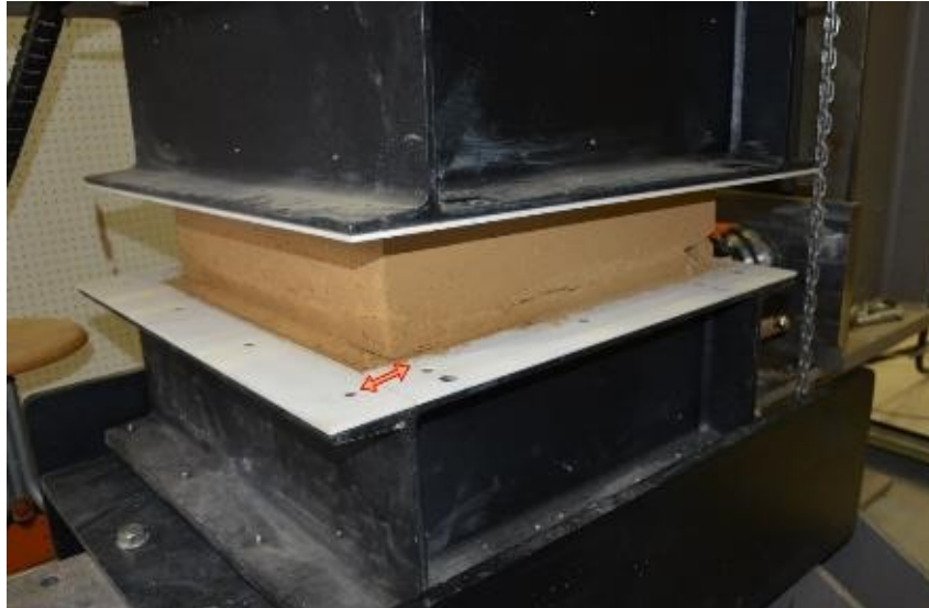
Figure 2.32 Unmolding of the upper part of the shear box after the test
