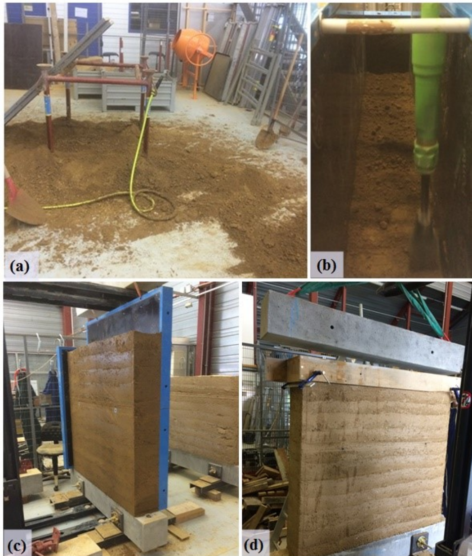
Figure 3.12 Manufacture of the wallet-specimens: (a) preparation of the soil; (b) compaction by the means of a pneumatic rammer; (c) demolding the frameworks; (d) placing the concrete beam on top of the wall
