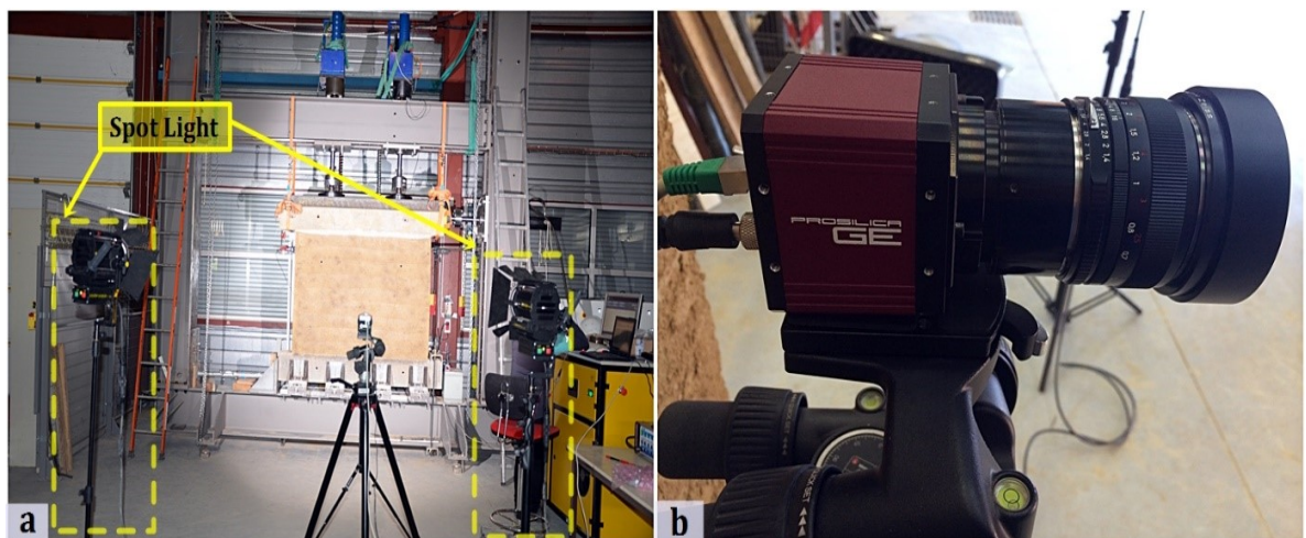
Figure 3.16 (a) The position of spot lights and camera; (b) Close-up of a camera and adjustment apparatus
