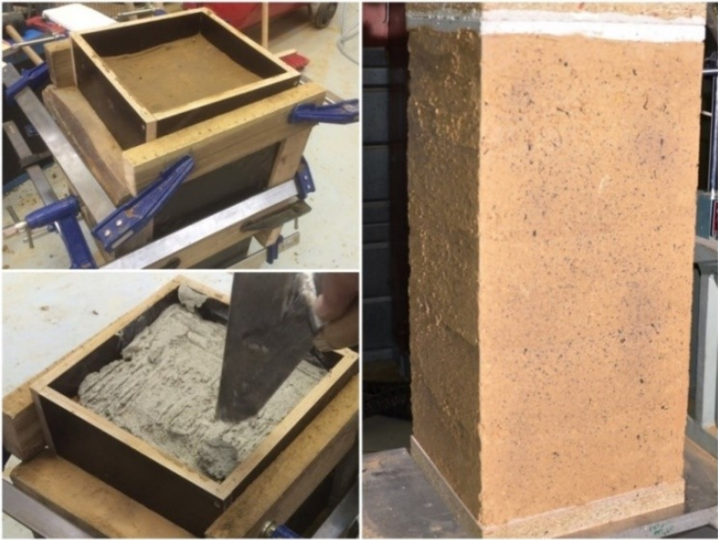
Figure 2.11 Prismatic specimens (25 cm × 25 cm × 50 cm) after surfacing
