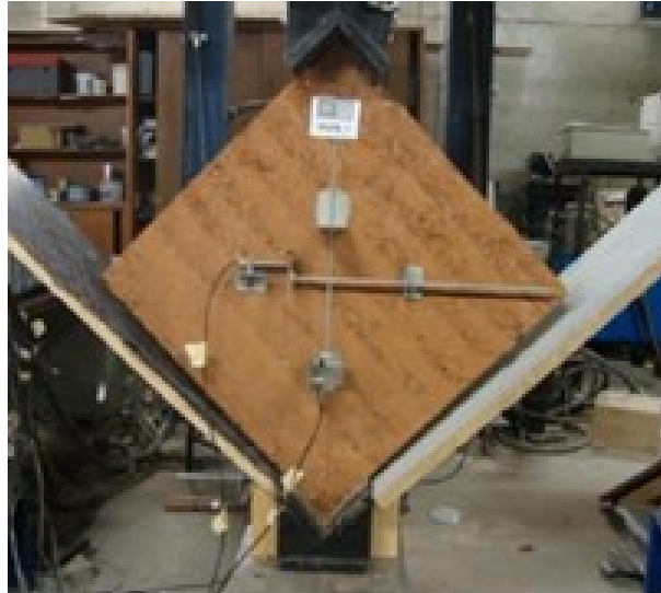
Figure 4.5 Experimental setup of a diagonal compression test [99]
