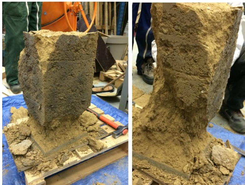
Figure 2.22 Failure of prismatic specimen
