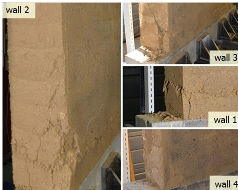
**Figure 3.31 Crushing on the left side for different walls during the test**
