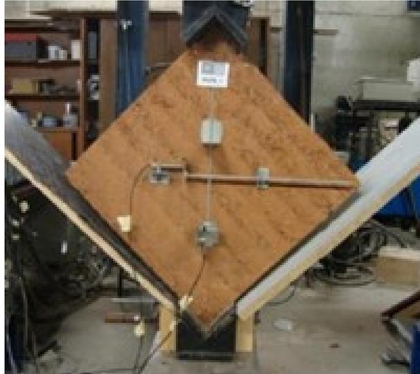
**Figure 4.5** Experimental setup of a diagonal compression test [99]
