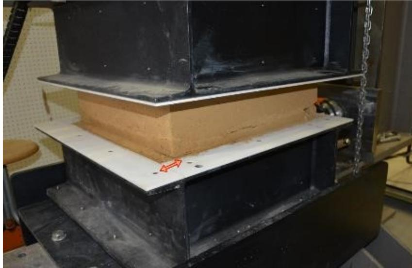
**Figure 2.32 Unmolding of the upper part of the shear box after the test**
