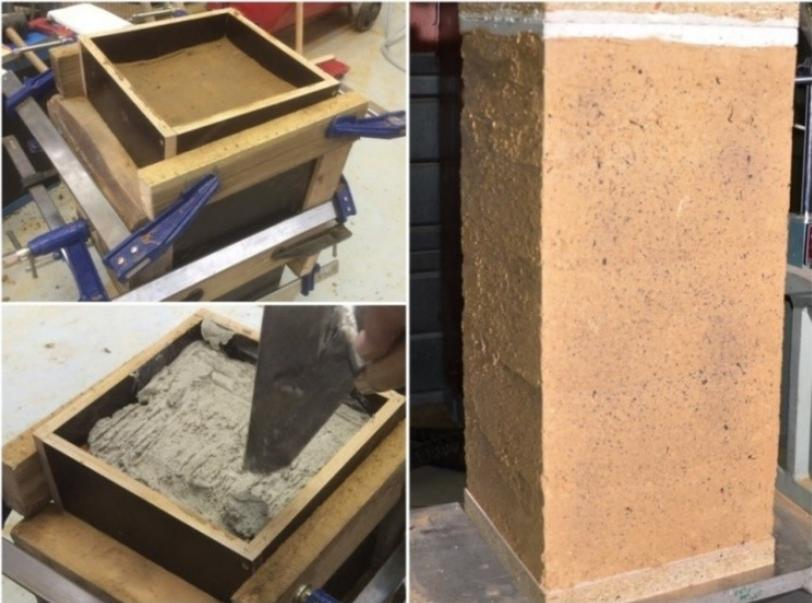
**Figure 2.11 Prismatic specimens (25 cm × 25 cm × 50 cm) after surfacing**
