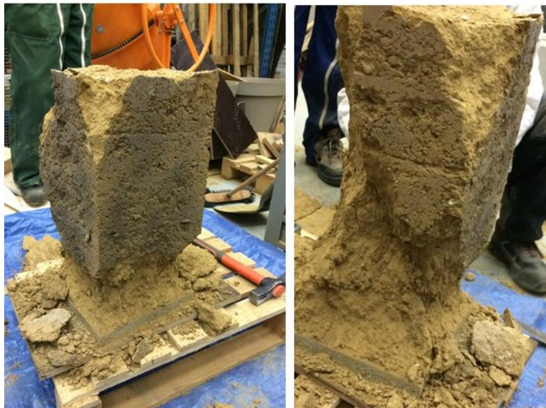
**Figure 2.22 Failure of prismatic specimen**
