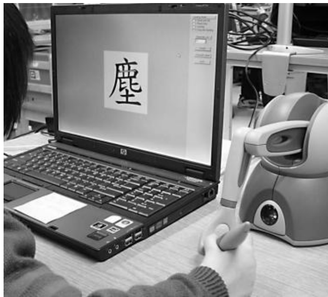
Figure [1.11]: The Phantom ®Omni® haptic device
