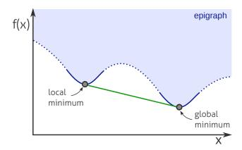
Figure 3.1: A function with multiple distinct minima cannot be convex. In the vicinity of a minimum the function can be approximated by a parabola (solid blue lines). Convexity requires every line connecting two point on the graph of the function to lie completely within the epigraph (light blue shaded region) of the function, *i.e.* above or on the graph. A line connecting two local minima (solid green line) cannot fulfill this requirement.
