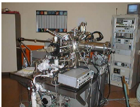
Figure 29: Scanning tunneling microscope, equipped for UHV experiments (CEA Saclay, IRAMIS Group)
