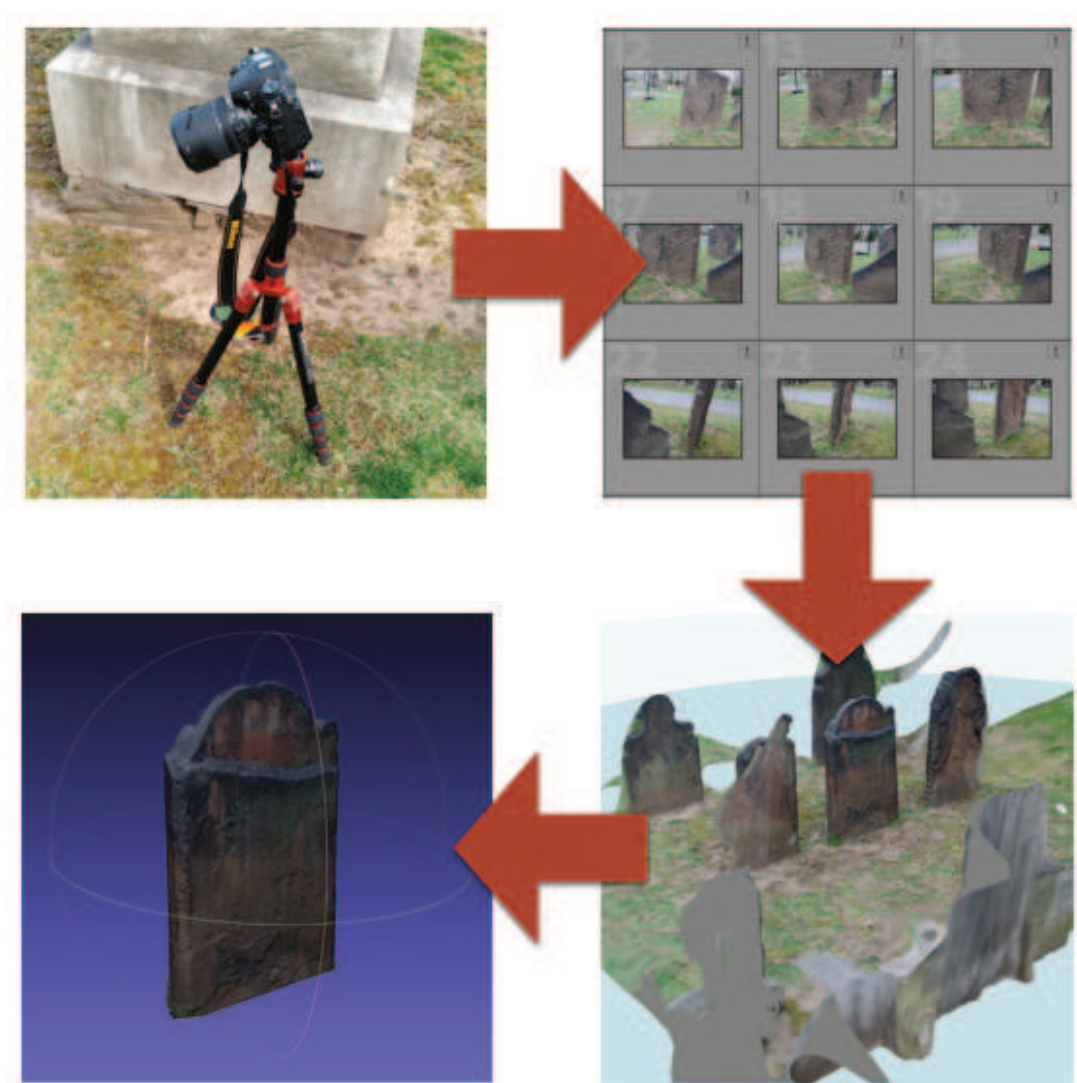
Figure V.2: Our method requires an isolated 3D manifold model to work properly. Generating it consists on taking pictures, loading them to Autodesk ReMake, which generates a 3D reconstructed scene and, then, separating the target model and filling its holes.
