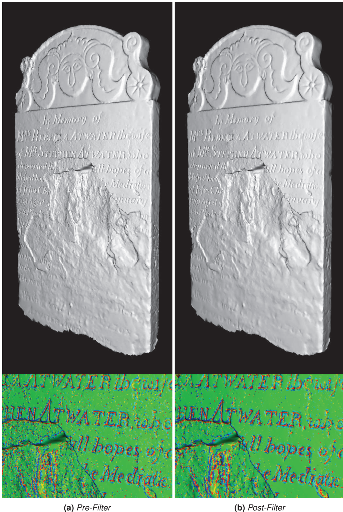
Figure V.3: We perform a smoothing filter to reduce the acquisition noise of the reconstructed model. Here it shows a comparison before and after applying the filter (top) and zoom-in's showing the obtained color-coded curvature in each case (bottom).
