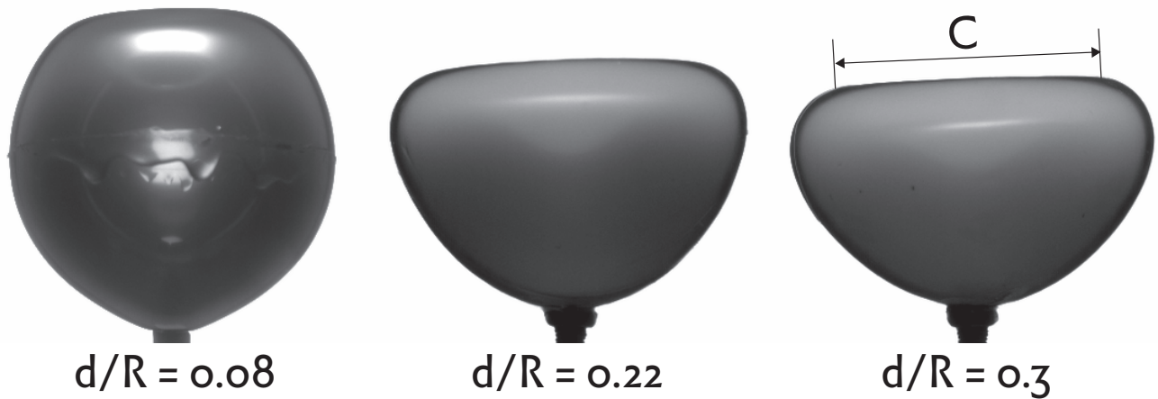
Figure 3.3: Shape after buckling for different \frac{d}{R} parameters, when submitted to external pressure variations. C extracted from connection points between external fit of the shape and fit of the concavity (see sec.2.2.4.2).
