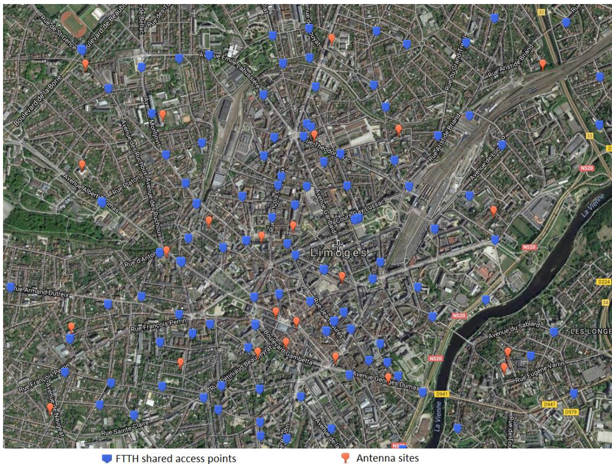
Figure V-12 : Geographical location of antenna sites and FTTH shared access points of the city of Limoges in France
