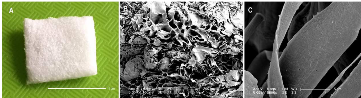
Fig. 1. Urgo resorbable bovine collagen I implant. (A) Macroscopic view. (B), (C) Scanning electron microscopy of the collagen implant. Scale bars = 1 cm (A); 200 \mu m (B); 5 \mu m (C).
