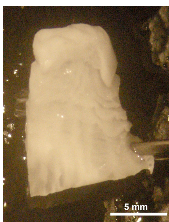
Figure 1. Light micrograph of 700 \mu\text{m} thick PCL (poly( \epsilon -caprolactone)) electrospun-nanofiber scaffold.
