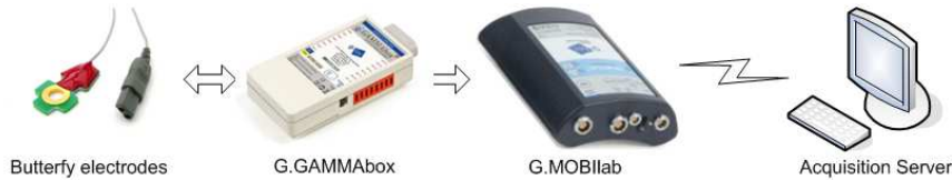
Figure 4.3: Acquisition material, the EEG is recorded with electrodes, the signal is amplified and sent to a computer running OpenVIBE.
