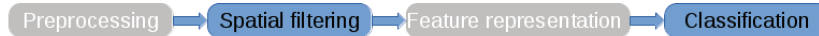
Figure 3.1: BCI signal processing pipeline. The fundamental blocks for machine learning are in blue ( i.e. spatial filtering and classification). Filters and classifiers are learned from training data. Gray blocks ( i.e. preprocessing and feature representation) do not require learning.
