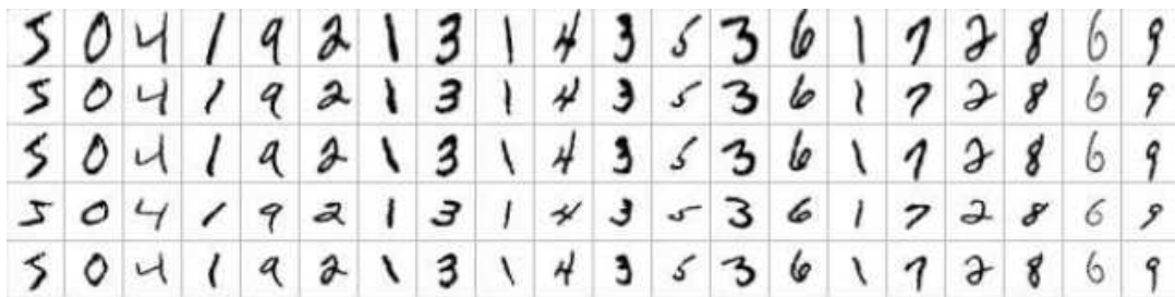
Figure 6.1: Hand-written digits from MNIST dataset. The original data are on the first row, the other rows are artificially created images from distorted version of the original digits. [Image taken from Ciresan et al., 2012]
