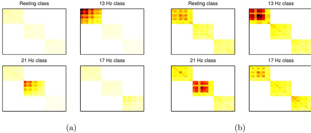
Figure 5.5: Representation of covariance matrices: each image is the covariance matrix mean  $\bar{\Sigma}^{(k)}$  of the class  $k$ , for one session of the recording. The diagonal blocks show the covariance in different frequency bands, i.e. 13 Hz in the upper-left block, 21 Hz in the middle, and 17 Hz in the bottom-right. Subjects with highest (a) and lowest (b) BCI performance.
